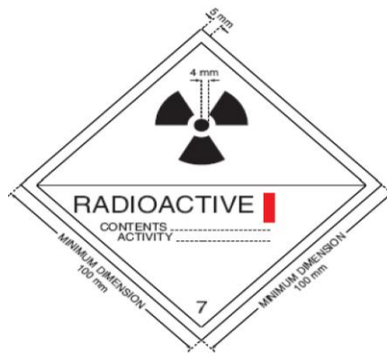
Figure 2. Category I-WHITE label. The background color of the label shall be white, the color of the trefoil and the printing shall be black, and the color of the category bar shall be red.
