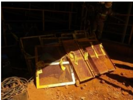
Improper – Not installed on a barricade post.
