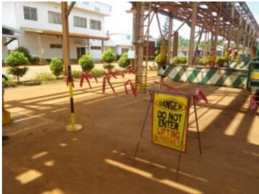
Proper- provided with post, indication tag and access way.
