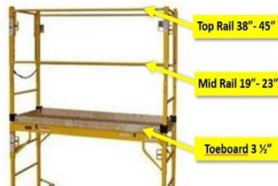
Fig. 2 Standard Guardrail
