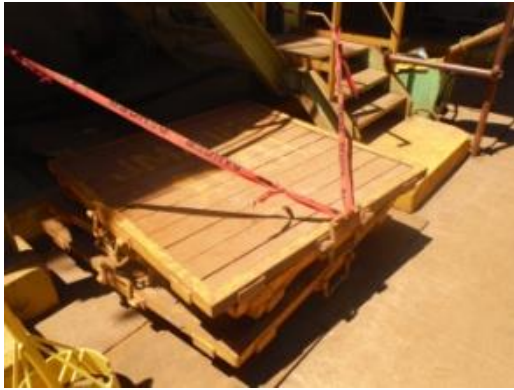
Improper – Should be caution tape only not danger tape. No barricade post
