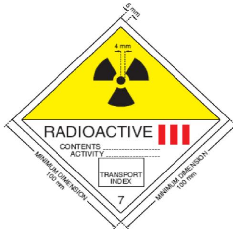
Figure 4. Category III-YELLOW label. The background color of the upper half of the label shall be yellow and the lower half white, the color of the trefoil and the printing shall be black, and the color of the category bars shall be red
