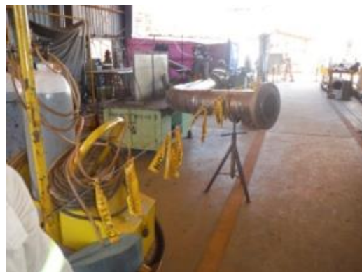
Improper – Barricaded parts extending outside.
